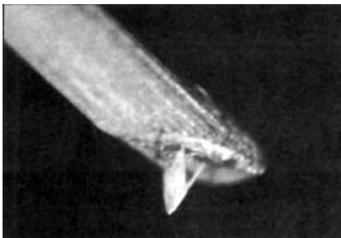
The mounted van den Hul tip and boron cantilever
